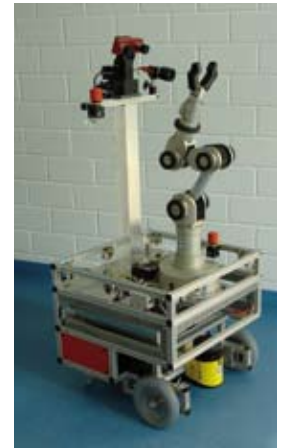
In 2007 b-itAS acquired a new robot platform with a 5 degree-of-freedom „Katana“ arm, including several sophisticated sensor systems and a powerful computing unit. The platform will serve for various projects concerning robot navigation and mobile manipulation.
