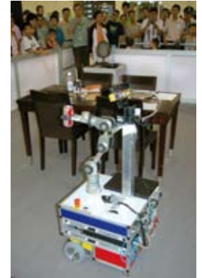
The b-itAS team at the RoboCup World Championships in Suzhou, China. In 2007 b-itAS acquired a new robot platform with a 5 degree-of-freedom Katana arm, including several sophisticated sensor systems and a powerful computing unit.
